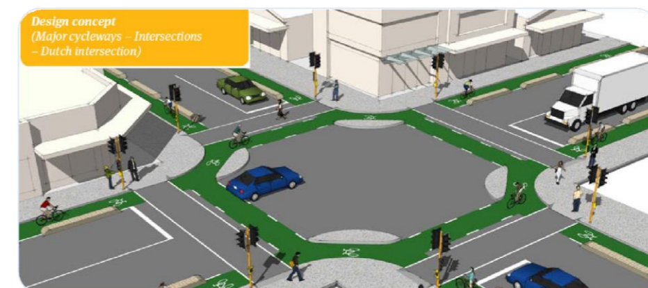
Figure 16: Key Infrastructure Elements of Protected Junction
